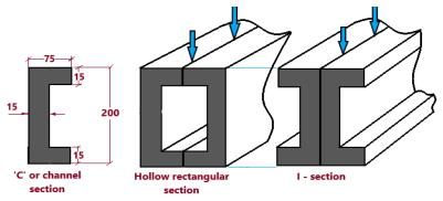
OR, Compare the bending strength of three sections of the same cross sectional area and depth if one of them has a solid rectangular section (50 mm wide and 200 mm deep), the second one is of hollow rectangular section (external dimensions of 90 mm wide and 200 mm deep with 20 mm wall thickness), and the last one is an I-section of equal flanges (170 mm wide web and flange thickness equal to 20 mm).
